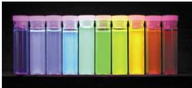
Fig. 4. Ten distinguishable emission colors of ZnS capped CdSe QDs excited with a near-UV lamp. From left to right (blue to red), the emission maxima are located at 443, 473, 481, 500, 518, 543, 565, 587, 610, and 655 nm [20].
