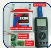
A system has been developed wherein the CO<sub>2</sub> gas sensor module detects gas and sends quantitative data to a digital multimeter (DMM). The DMM then sends data wirelessly to an Android app enabled mobile phone using a Bluetooth dongle. The data generated is also logged into a laptop using RS – 232 interface.
